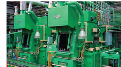
Heat-treatment furnace installed with a single-end radiant-tube burner
