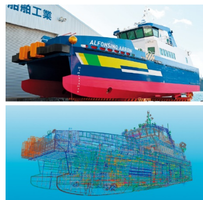
Crew transfer vessel Comparison of actual ship photo (top) and 3D model (bottom)
