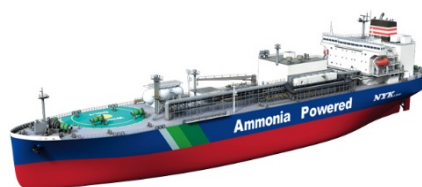
Ammonia-fueled medium gas carrier CG image
