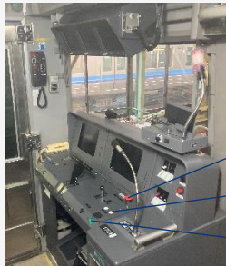
▲ Driver's cab equipped with automated operation system
