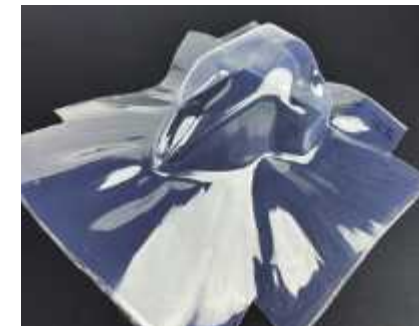
The features of the ultra-high-rigidity biaxially oriented polypropylene sheet (new OPP) under development include its formability and transparency, and that it can be decorated
