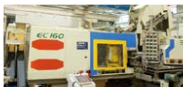
Four-color injection molding machine that is currently in use (multicolor molding machine)
