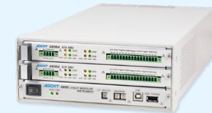
Capable of battery emulation 4-channel source monitor unit
