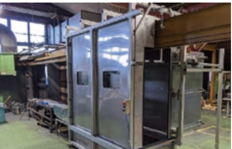
Reduction of dichloromethane using in-house designed and manufactured cleaning unit
