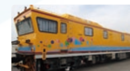
Ultrasonic rail inspection cars that use ultrasonic waves to detect flaws inside rails
