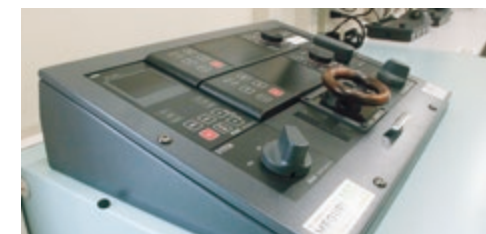
Autopilot system aboard an experimental fully autonomous ship
