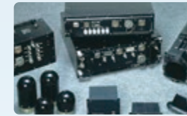
Radar warning receivers for aircraft that warn pilot of threat radar signals
