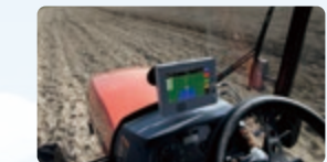
Automatic control system enabling agricultural vehicles to automatically drive straight
