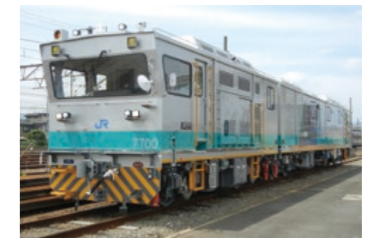
The company's core product: Ultrasonic rail inspection car
