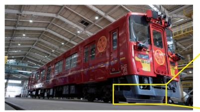
A multifunction inspection car of Kyushu Railway Company (JR Kyushu) equipped with the track diagnosis support system
