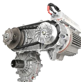
CVT drive unit integrating transmission functions developed by our company
