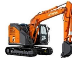
Hitachi Construction Machinery: 13-ton class electric hydraulic excavator ZX135-7EB
