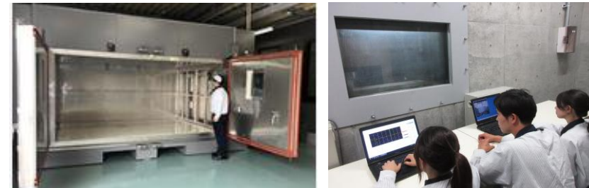
Capable of performing various safety tests for secondary batteries compliant with United Nations regulations and other standards Battery Safety Testing Center
