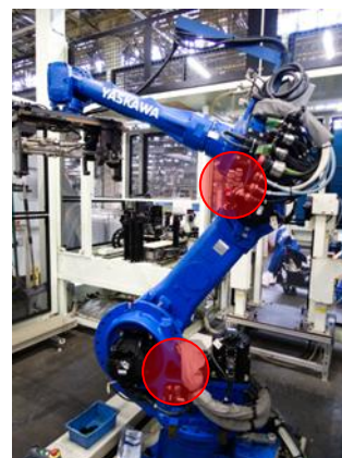
Power module equipped with Maxell's All-Solid-State Batteries Industrial Robot Equipped with All-Solid-State Batteries (Power Module Installed at the Location Indicated by the Red Circle* 1 )
