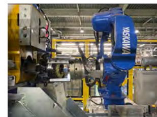
The multi-axis robotic arm automates the cutting/recovery process
