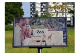
Reflective IGZO display with high outdoor visibility
