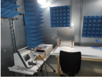
Static electricity testing environment in shielded room
