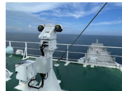
Outdoor surveillance using an ultra-high-sensitivity camera mounted on a pan-tilt platform
