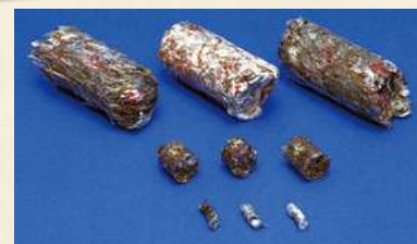
RPF (refuse paper and plastic fuel), an alternative fuel
