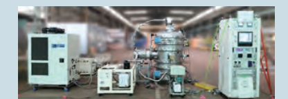
Vacuum exhaust prototype for liquefied hydrogen storage tank
