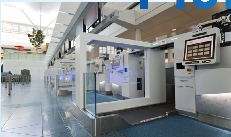
A self-service baggage drop unit equipped with facial recognition system delivered to Haneda Airport
