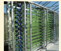
Microalgae cultivation facility (sealed glass tubes type photobioreactor)
