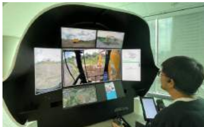
Smart Construction Teleoperation cockpit
