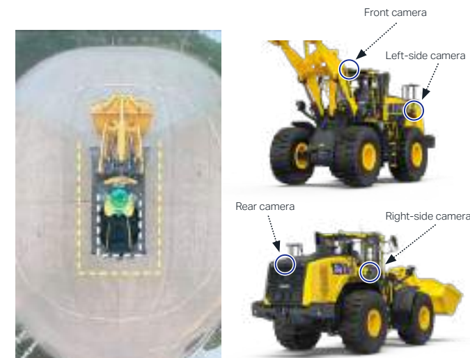
Bird's-eye view image and installed cameras of the WA470-11 wheel loader
