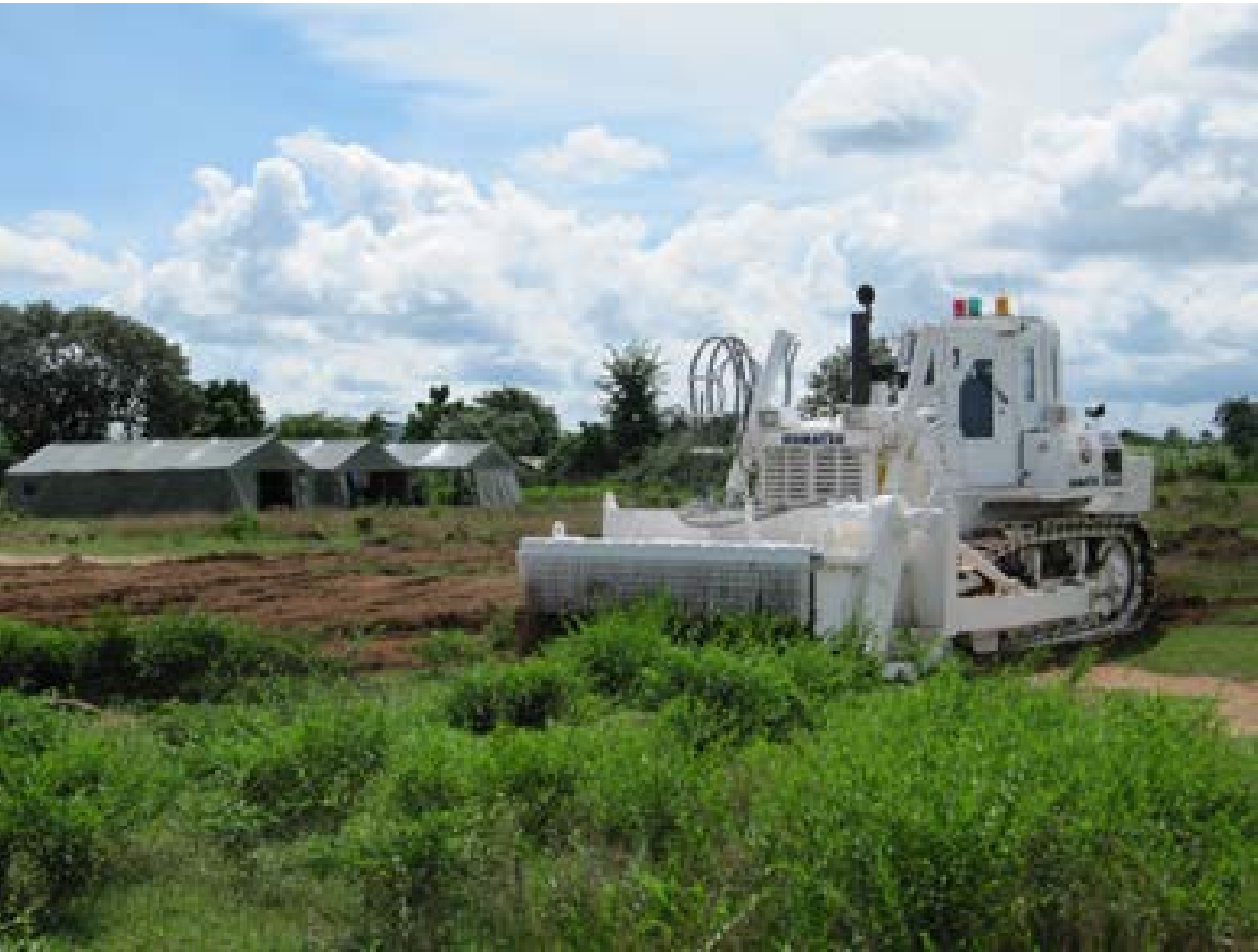
A D85MS-15 anti-personnel landmine clearance machine operating in Cambodia
