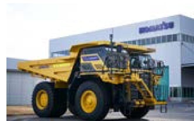
Concept machine of a large dump truck equipped with a hydrogen combustion engine
