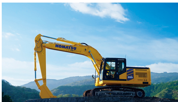
[PC200i-12 hydraulic excavator equipped with 3D machine guidance as standard]
