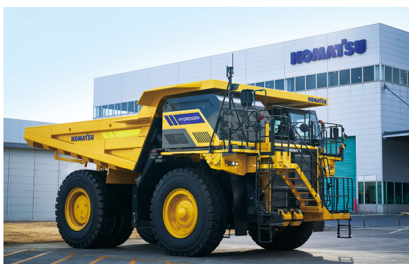
[Concept machine for the HD785 large dump truck equipped with a hydrogen combustion engine]
