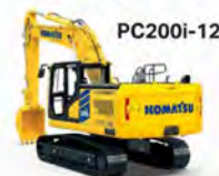
PC200i-12 New-generation hydraulic excavator, 3D machine guidance as standard feature
