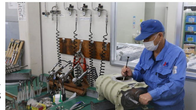
A technician overhauls a pump
