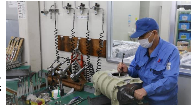
A technician overhauls a pump
