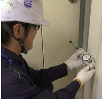
Legal inspection of fire doors
