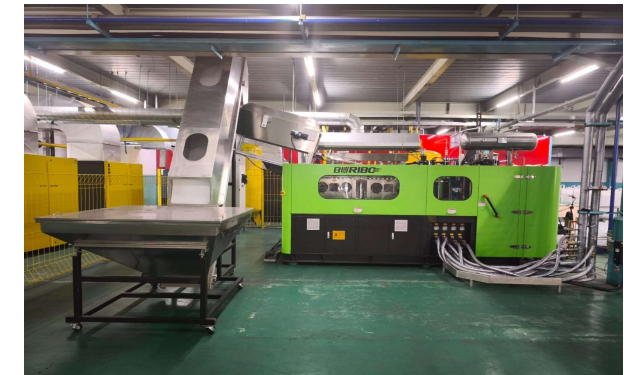
PET gallon bottle blow-molding machine
