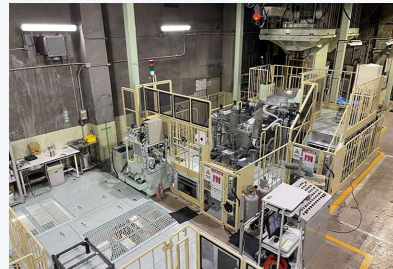
Vertical high-speed twin-roll caster prototype (R&D Center: Nagoya)
