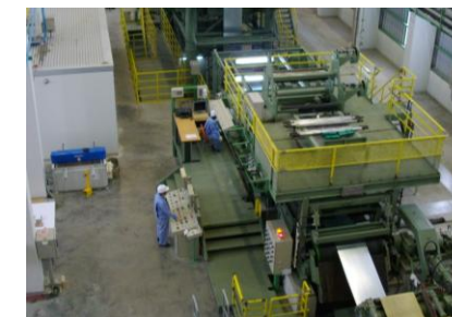
Continuous coating line
