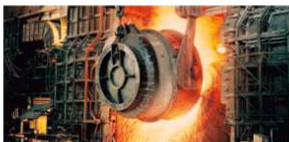
JFE Steel Corporation West Japan Works (Kurashiki) converter
