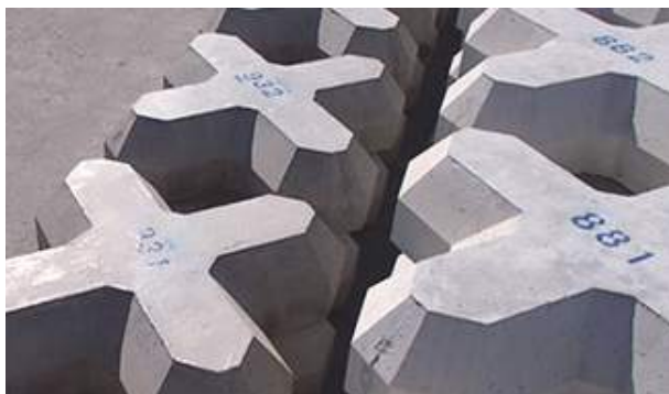
Wave-dissipating and foot protection block
