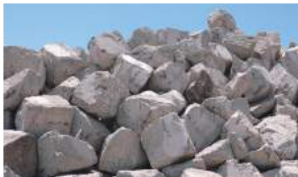
Artificial stones made from steel slag hydrated matrix
