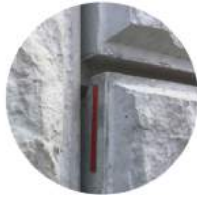
Fail-Sensor indicator (red indicating internal anomalies)
