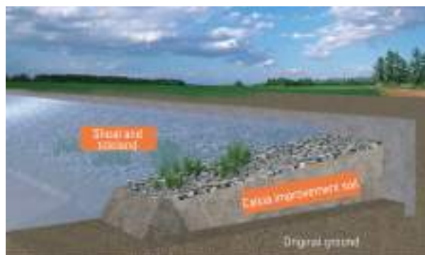
Example of calcia improvement soil application (shoal and tideland construction material)
