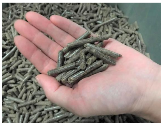
EFB pellets (produced by PTEC)
