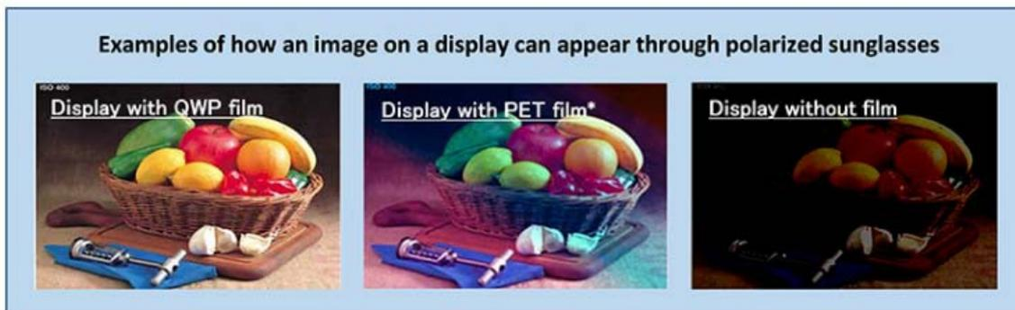
The image of the "Display with PET film" is an example of how an image can appear when PET (polyethylene terephthalate) film is applied on a display in place of QWP film.
