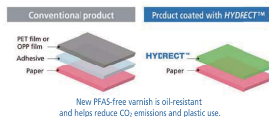
Laminated packaging material coated with water- and oil-resistant HYDRECT varnish
