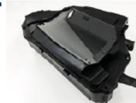
Automotive HUD with optical sheet
