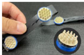
Soft-dry electrodes made of resin (hydrogel type)
