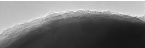
Silica treatment layer of conventional titanium dioxide
