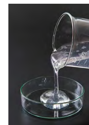
CNF: An innovative material made from wood-derived fiber micro-refined to the nano level
