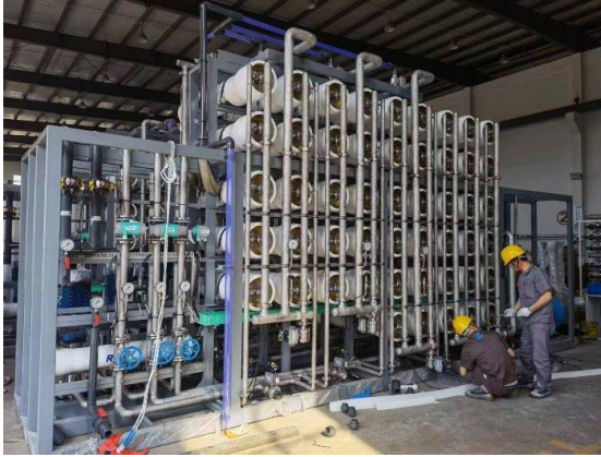
BC membrane installed concentration equipment For Lithium recovery, wastewater treatment, etc.
