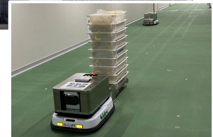
Automated guided vehicle (AGV) for transporting semi-finished products in a plant
