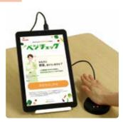
A device that measures estimated vegetable intake volume simply by holding the palm of your hand over a sensor for about 30 seconds
