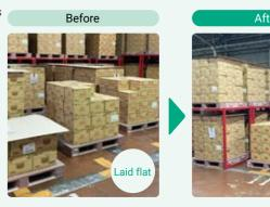
Utilizing space more effectively by switching from laid flat to steel pallets (Ueno Plant)
