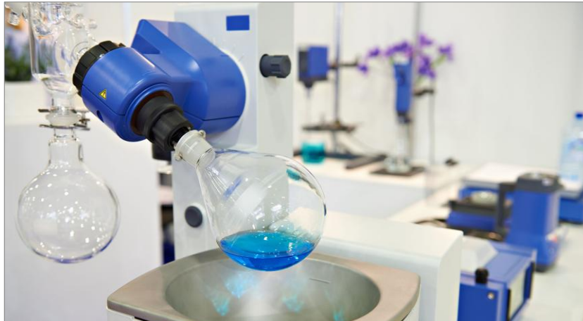
Reagent concentration by evaporator
