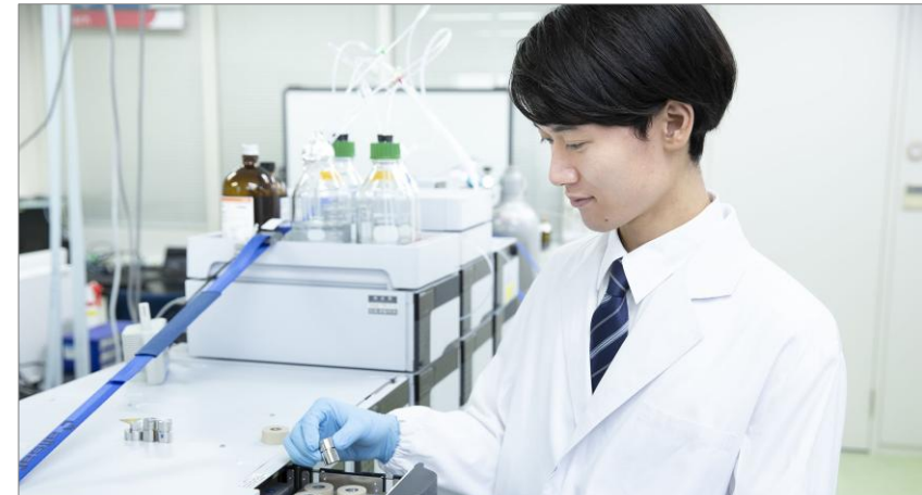
Component analysis by HPLC
