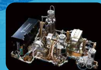
Lunar water electrolysis equipment aboard the lunar lander
