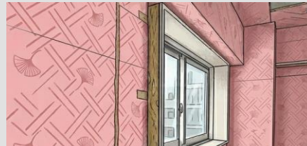
Renovated condominiums (phenolic foam boards)
